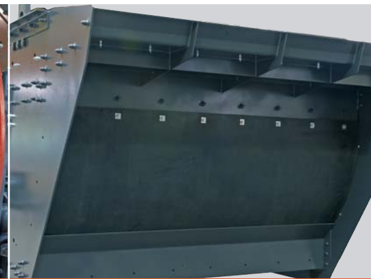
Dust encapsulation in feed end
