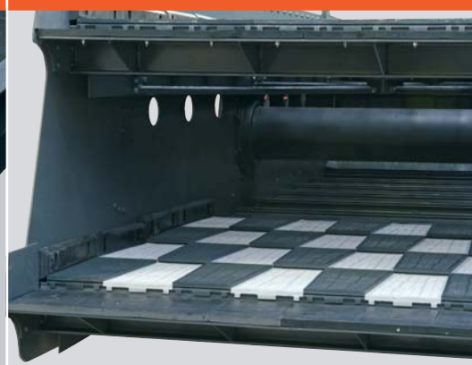
Adapted for all screen media thanks to modular deck design and adapters
